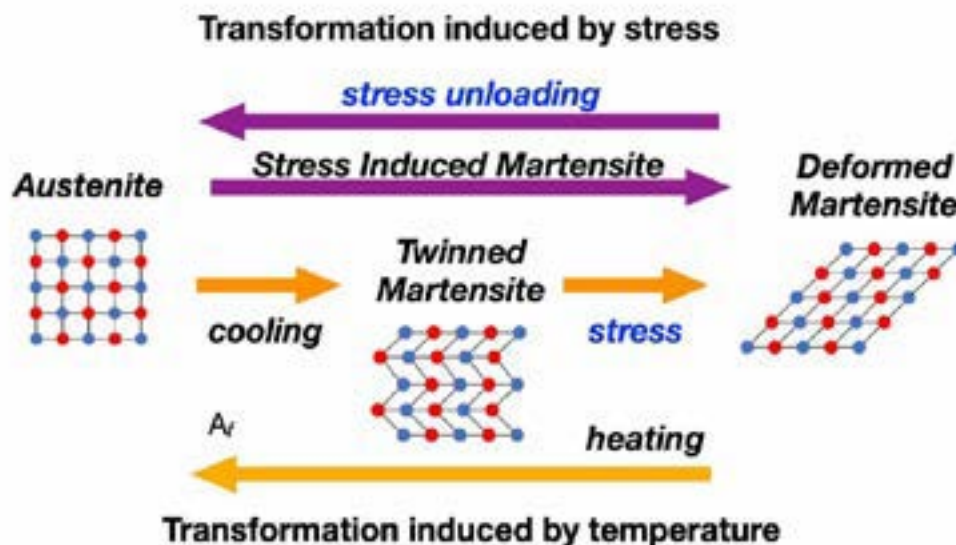
Figure 4. Schematic representation of phase crystallographic transformation of NiTi alloy induced by stress or temperature
