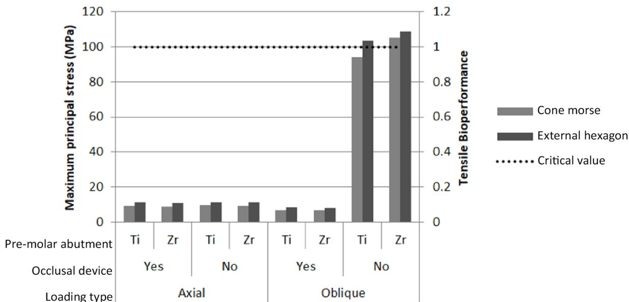
Figure 3: Maximum tensile stresses at bone tissue and tensile bioperformance.
