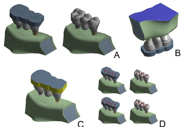
**Figure 2:** Representative finite element models: a) Mesh; b) Fixed constraints in blue; c) Vertical movement allowed at occlusal device (restrictions at yellow surface); d) Loading conditions.
