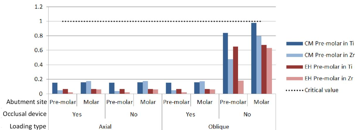
**Figure 9:** Stress ratio at abutments. Ti and Zr indicate the material of pre-molar abutment. Ti abutments were evaluated by von Mises stress ratio, Zr abutments were evaluated by maximum principal stress ratio
