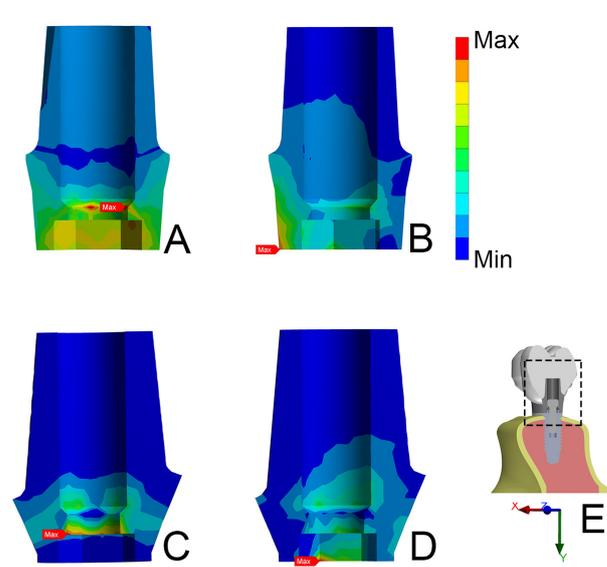
**Figure 11:** Stress field at EH pre-molar abutments. A) Ti abutments, all axial loadings and oblique loading with occlusal device; B) Ti abutment, oblique loading without occlusal device; C) Zr abutments, all axial loadings and oblique loading with occlusal device; D) Zr abutment, oblique loading without occlusal device; E) Viewpoint.
