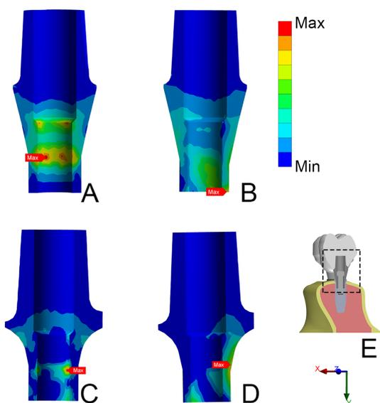
**Figure 10:** Stress field at MT pre-molar abutments. A) Ti abutments, all axial loadings and oblique loading with occlusal device; B) Ti abutment, oblique loading without occlusal device; C) Zr abutments, all axial loadings and oblique loading with occlusal device; D) Zr abutment, oblique loading without occlusal device; E) Viewpoint.
