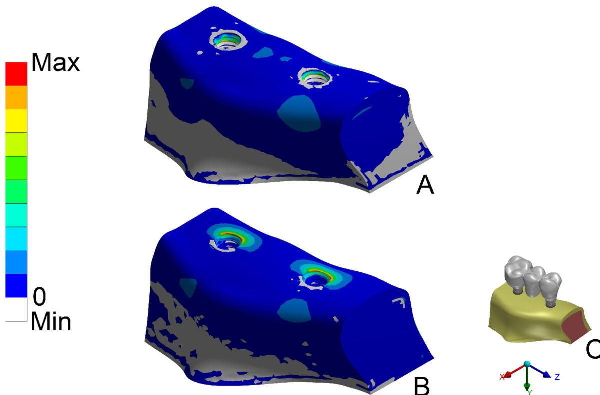
Figure 4: Tensile stresses fields at bone tissue. A) All groups with axial loading and the oblique loading with occlusal device; B) Oblique loading without occlusal device; C) Viewpoint.
