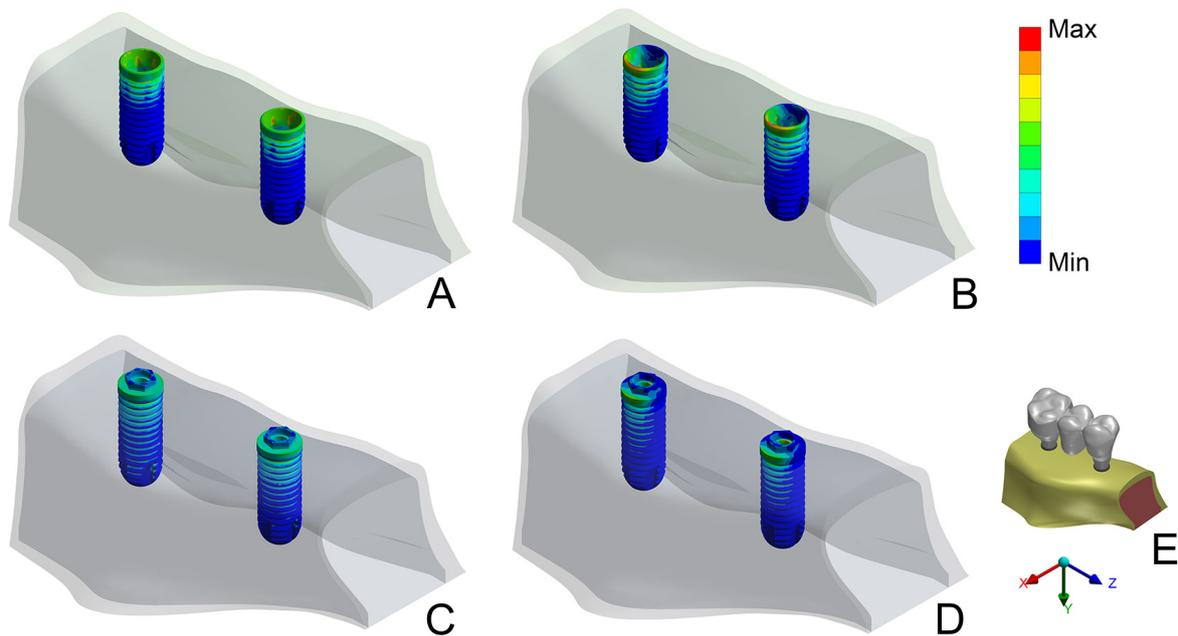
**Figure 8:** Von Mises stresses fields at implants. A) MT implants, all axial loadings and oblique loading with occlusal device; B) MT implants, oblique loading without occlusal device; C) EH implants, all axial loadings and oblique loading with occlusal device; D) EH implants, oblique loading without occlusal device; E) Viewpoint.
