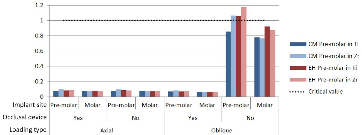
**Figure 7:** Von Mises stress ratio at implants. Ti and Zr indicate the material of pre-molar abutment.
