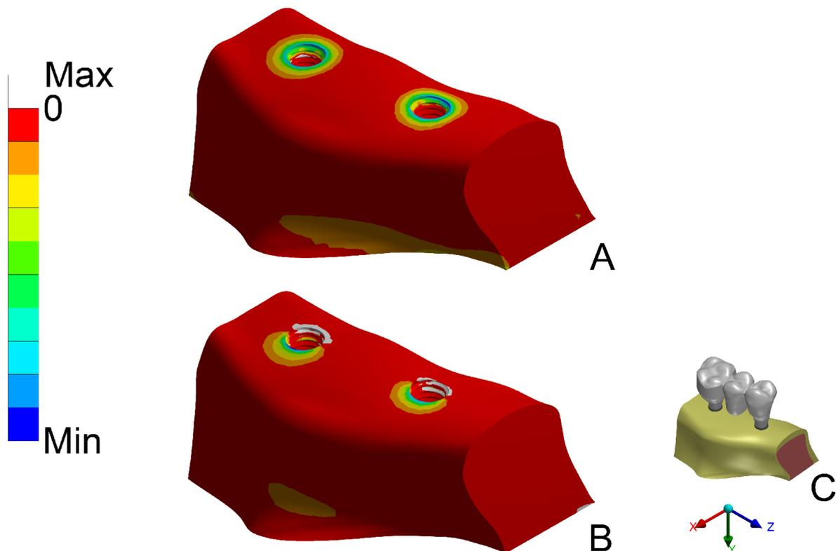
Figure 6: Compressive stresses fields at bone tissue. A) All groups with axial loading and the oblique loading with occlusal device; B) Oblique loading without occlusal device; C) Viewpoint.
