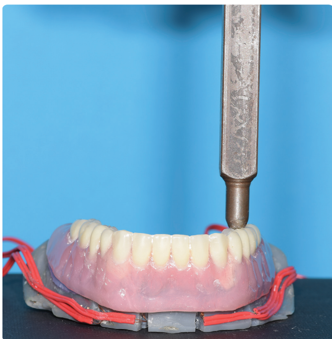
Figure 4: Unilateral load of 100 Newton (N) was applied on the central fossa of the mandibular left first molar using I bar applicator of the Universal testing machine
