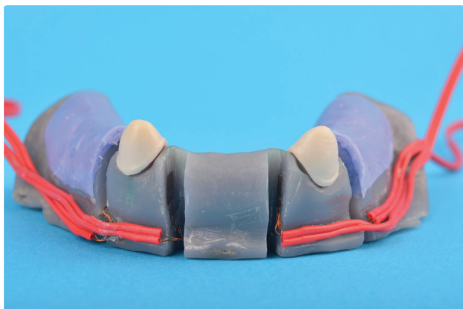
Figure 3: Strain gauge rosettes were bonded on the mesial and distal sides of both abutments using cyanoacrylate adhesive
