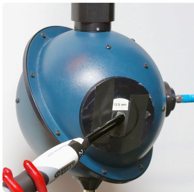
Figure 1: Bluephase Style lights measured using a 6" integrating sphere attached to a fiberoptic spectrometer
