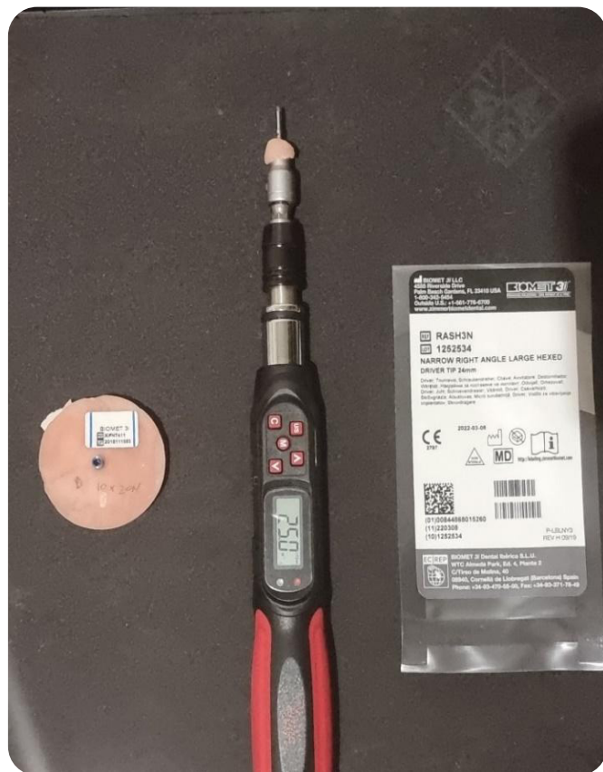
Figure 3: a) Implant fixed in self-curing acrylic; b) Screwdriver used to untighten and determine the RTV.
