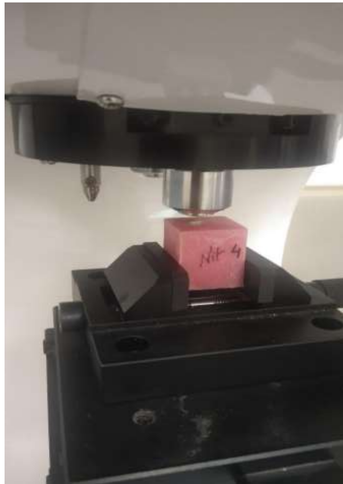
Figure 5: Close-up view of specimen positioning under the Vickers indenter during microhardness testing
