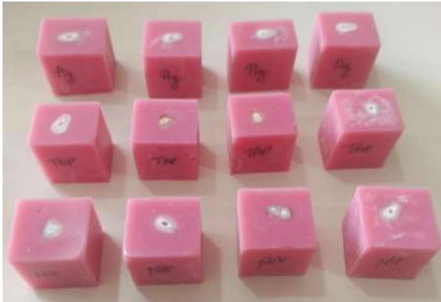
Figure 4: Distribution of acrylic-embedded root specimens into experimental groups: silver nanoparticles with chlorhexidine (AgNP+CHX), nitrofurantoin (Nif), and triple antibiotic paste (TAP)
