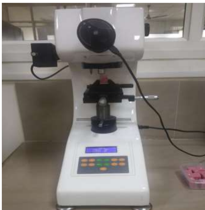
Figure 1: Vickers microhardness testing machine used for evaluating dentin microhardness of the specimens Sample Size Determination
