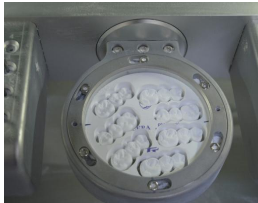
Fig:8 Milling of 3-unit monolithic bridges
