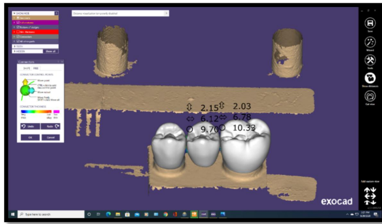
Fig: 7 CAD designing of 3-unit monolithic bridge connector dimension of 2(H) mm*6(W)mm
