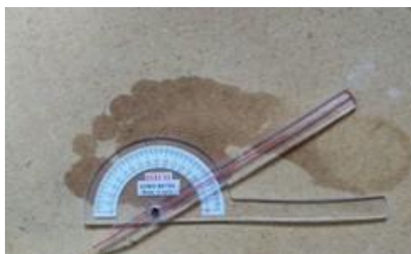
Fig.6: Goniometer used to measure the Clarke's angle
