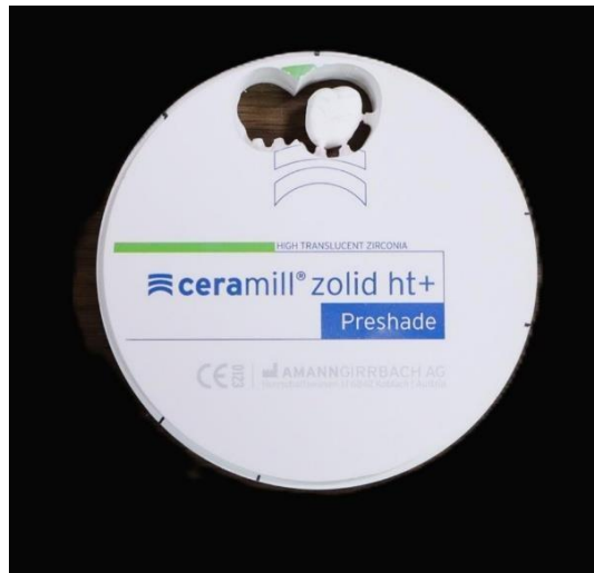
Figure 1 –Blank of Zirconia (AmannGirbach Ceramill® CAD/CAM Material – Zolid HT+ 14mm)
