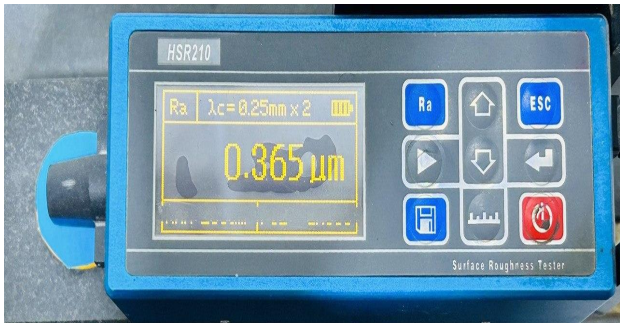
Figure 1: contact profilometer (surface roughness tester).
