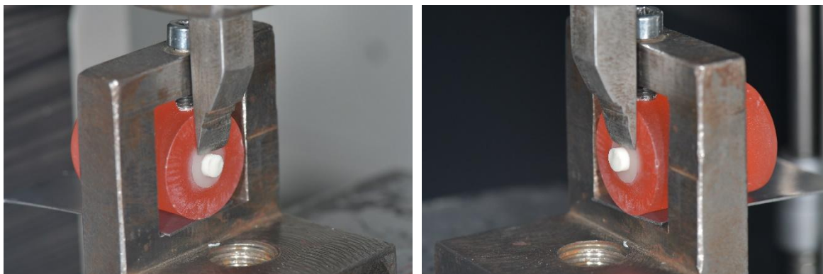
Fig.4 The specimen during the shear bond strength test
