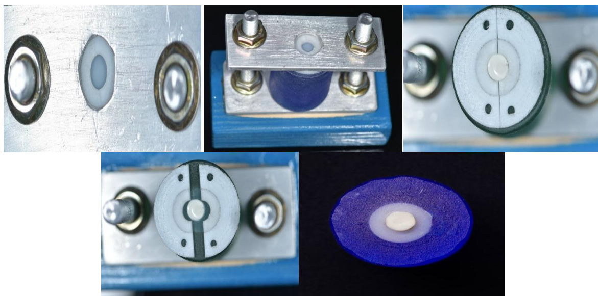
Fig.3 Custom-made split mold for application of resin cement
