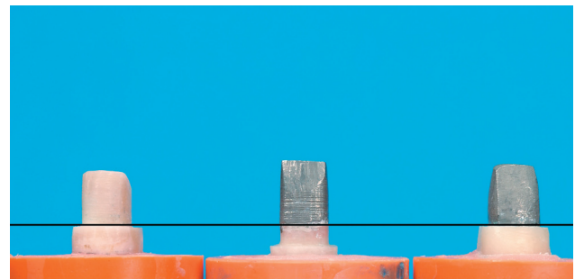
Figure 1. Photograph of mounted teeth, all dentine preparation, core plus ferrule, core without ferrule (L to R). Horizontal line indicates height above cemento-enamel junction.
