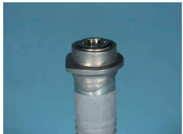
Figure 4. Coping was cast with grade 3 CP titanium.
