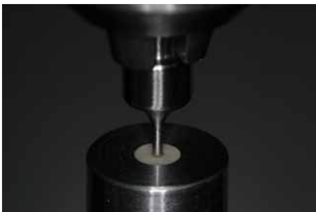
Figure 3. Push-out pin design.
