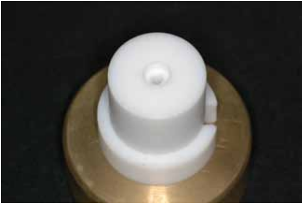
Figure 1. Cylindrical brass base and the white polytetrafluoroethylene system.
