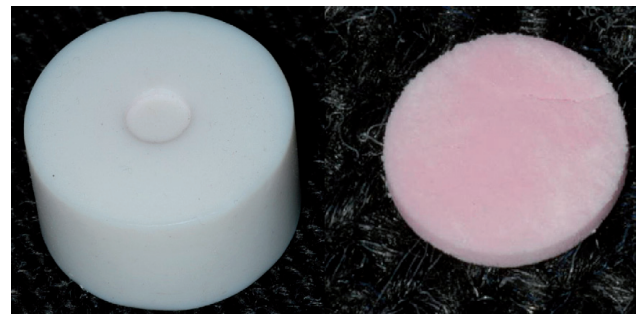
Figure 1. Shows the teflon mould with a porcelain disc.
