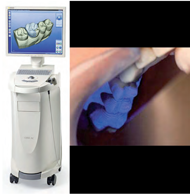
Figure 2. The Cerec® AC imaging unit. (2a) BlueCam camera (which uses a shorter wavelength blue light source via active triangulation sampling) and separate milling unit MC XL. (2b) Image of the prepared tooth captured using the Cerec AC BlueCam camera (figures retrieved from promotional site on Internet).
