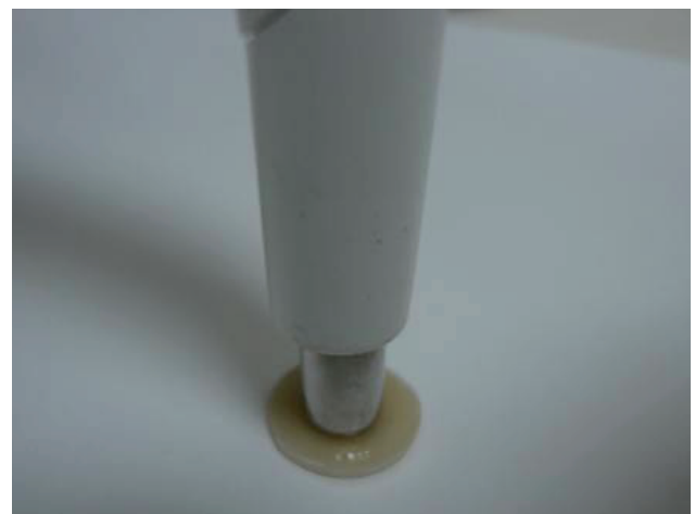
Figure 2. The colorimeter tip was placed in the center of each specimen with the glazed surface facing up against a white background.
