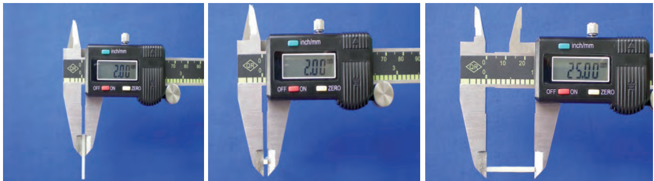
Figure 2. Dimensions of the Specimen (25 x 2 x 2 mm)
