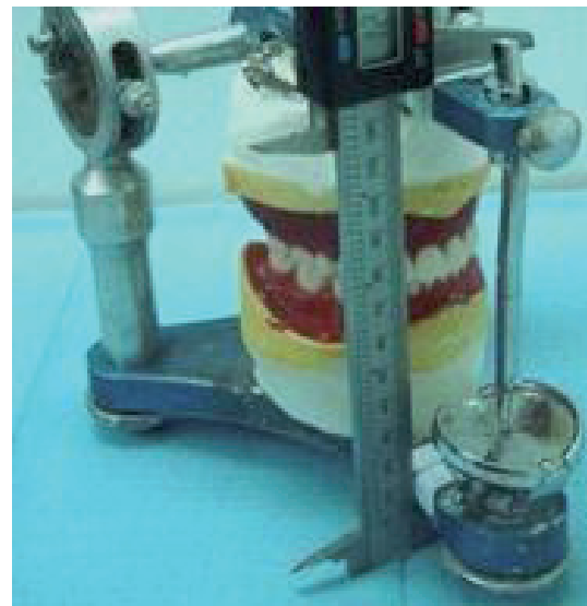
Figure 2. Measurement of the vertical dimension between the upper and lower arms of the articulator.
