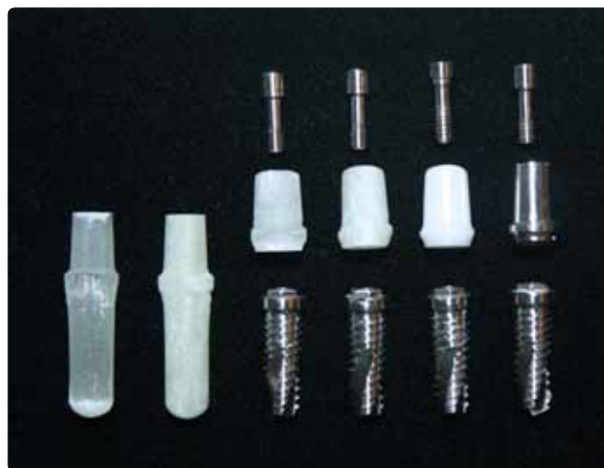
Figure 1: Representative images of the experimental groups, left to right: one-piece unidirectional FRC implant; one-piece bidirectional FRC implant; unidirectional FRC abutment; bidirectional FRC abutment; zirconia abutment; titanium abutment.
