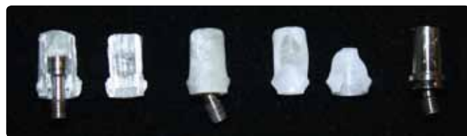
Figure 4: Representative fracture patterns of the abutments, left to right: unidirectional FRC; bidirectional FRC; zirconia; and titanium.
