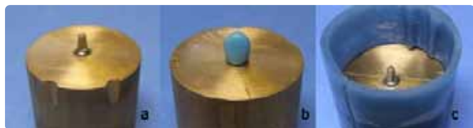
Figure 1: a) Implant fixture and ITI Straumann Solid abutment embedded into brass cylinder with 2 location notches to allow reproducibility. b) Canine tooth waxed up over abutment. c) Cylinder from light cured composite tray material made to fit accurately around brass casting including 2 location lugs on the internal surface.
