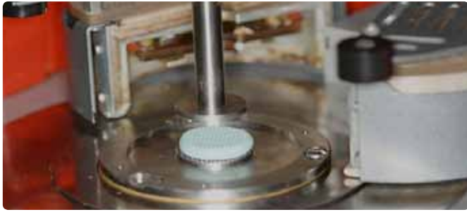
Figure 1: Sample in the rheometer chamber after 400 seconds test.
