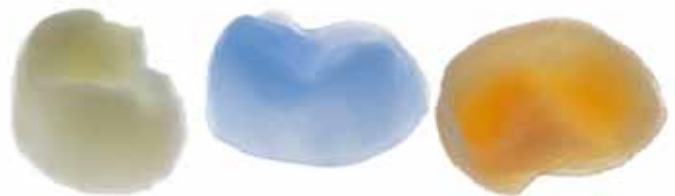
Figure 3: Handmade (white), milled (blue) and 3D printed additive manufactured (yellow) pattern for the onlay restoration.
