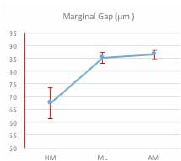
Figure 7: Mean of the marginal gap of the handmade (HM), milled (ML) and additive manufactured (AM) groups.
