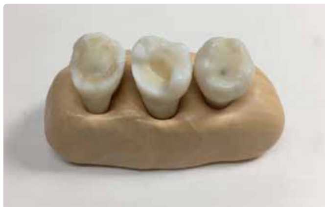
Figure 2: Representation of the teeth and putty block set-up. For digital copying, the teeth were inserted into putty blocks.
